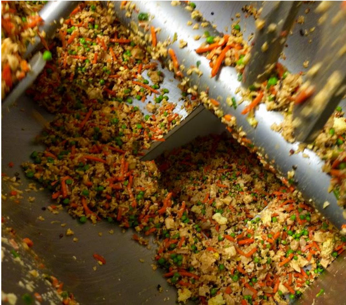
The tumbler's 400-pound capacity mixing tank empties through a pneumatic "trap door" in the bottom.
