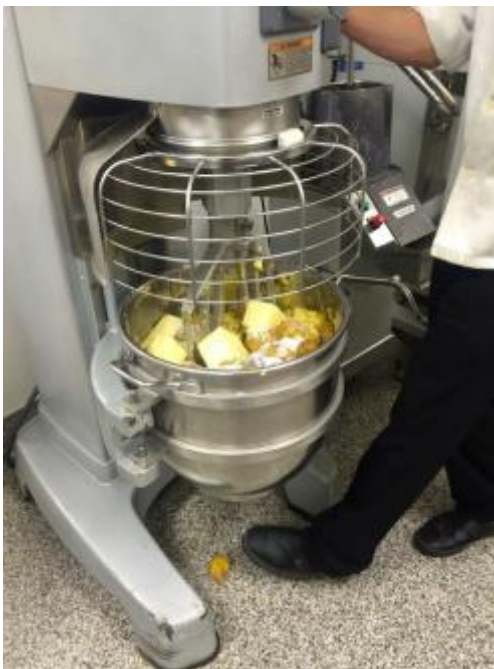
Making mashed potatoes the "old way," making several batches in 75-pound capacity Hobart mixers.
