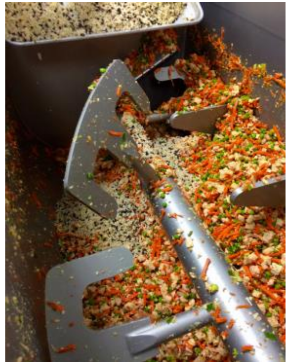
Variable-speed mixing arms gently toss fresh vegetables and other ingredients to make a more consistent, better-quality Thai Fried Rice.
